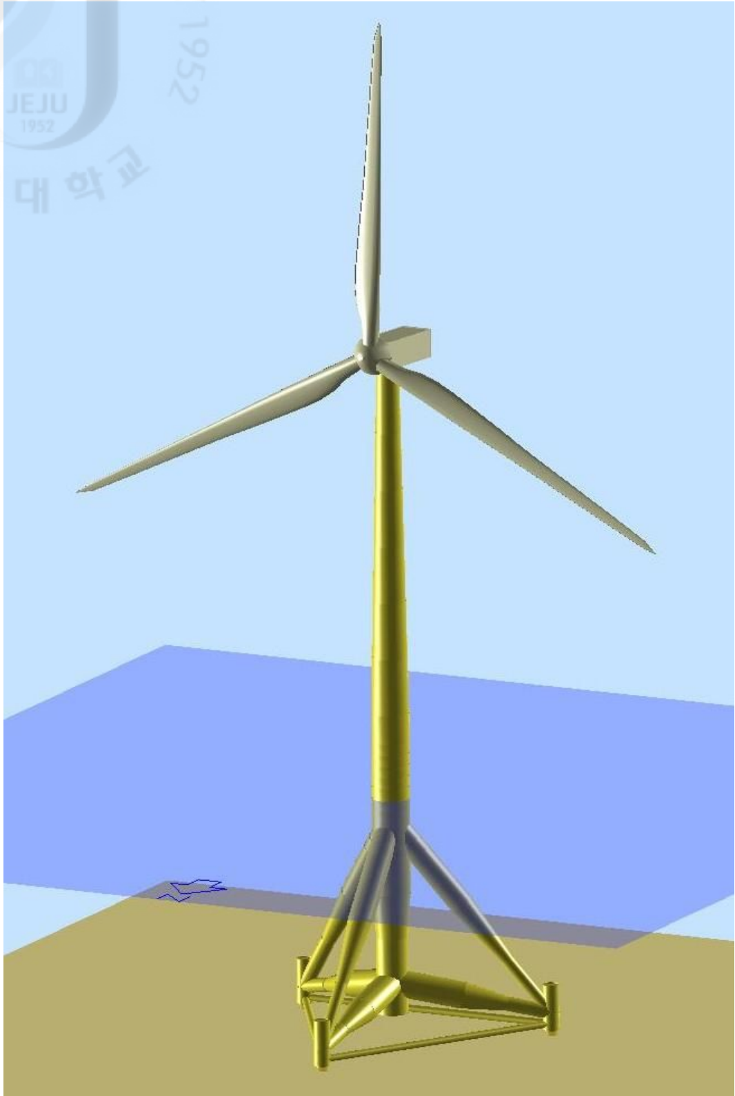
Fig. 16 Figure of 5MW tripod offshore wind turbine
