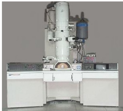
Fig. 16. Transmission electron microscope (JEOL, EM-2010).
