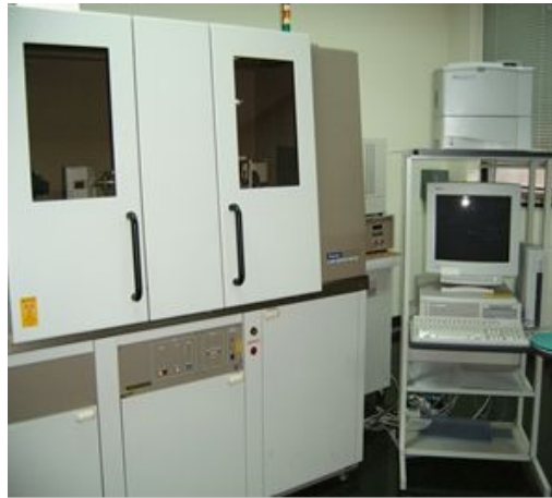
Fig. 17. X-ray diffraction analyzer (Rigaku Instruments C., D/MAX2200H).
