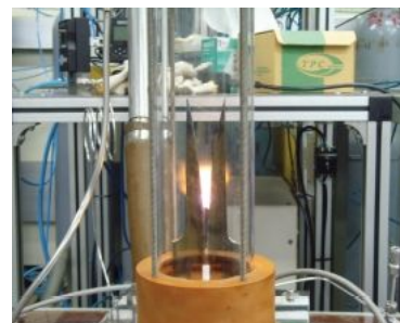
Fig. 4. Example of gliding arc plasma[19].
