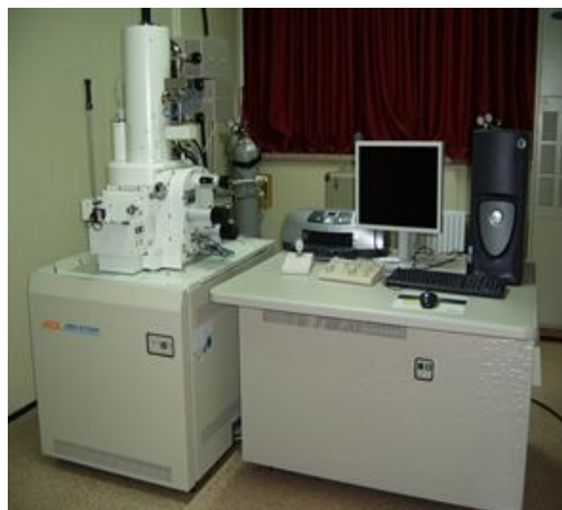
Fig. 15. Field emission scanning electron microscopy (JEOL Ltd., JSM-6700F).
