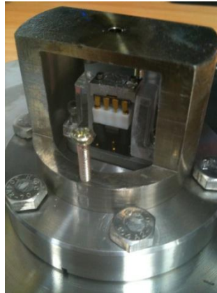
Fig 19 Mounted collimator at Feed-through
