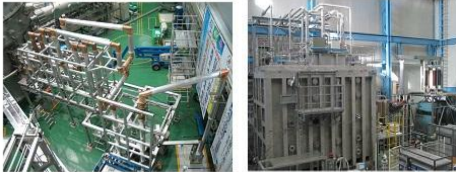
Fig 8 ICRF antenna and NBI for KSTAR
