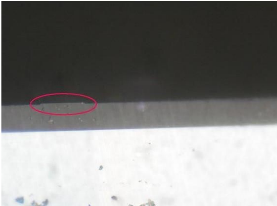
Fig. 28. Microscopy image of waveguide after lithography with polishing(show the ridge type waveguide in ellipsoidal).
