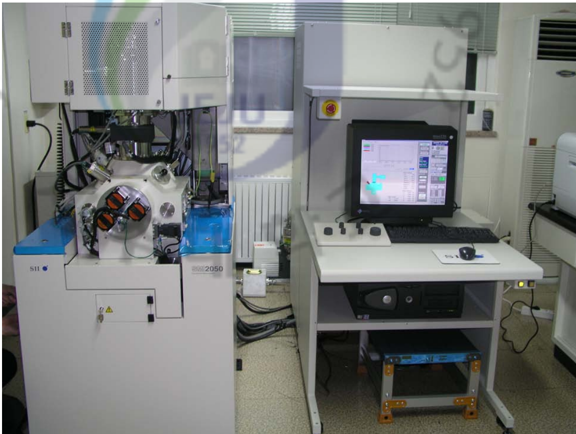
Fig. 3.1 A picture of FIB machine (SII NanoTechnology SMI2050) in Research Institute of Center (RIC).
