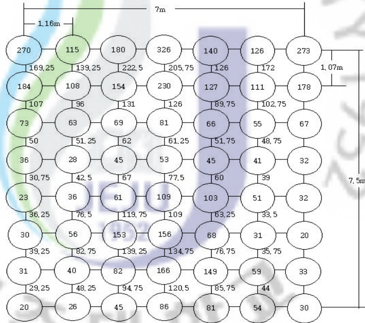
Fig. 21 The vertical illuminance values on 85cm by mock-up(2)
