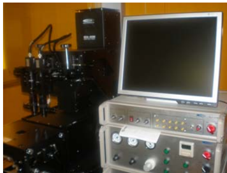
Figure. 3 Mask aligner system (MDA-400 M) for lithography pattern fabrication
