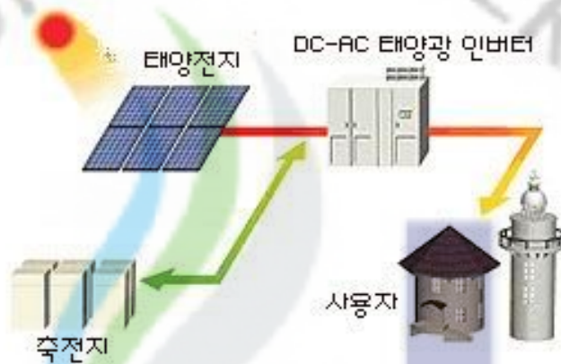
Fig. 5 Stand-alone PV system
