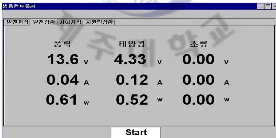
Fig. 41 Monitoring of power output for wind and PV generators
