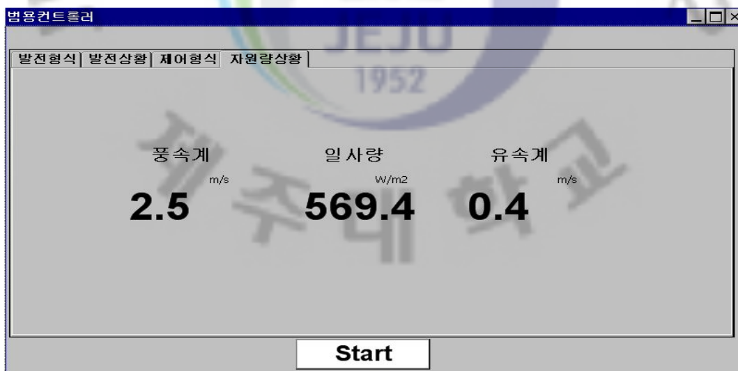
Fig. 45 Monitoring of wind, PV, tidal resources
