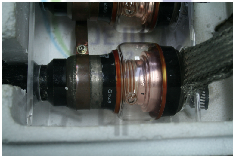
Fig. 30 Picture of the variable capacitor.
