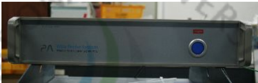
Fig. 39 DC power supply for electric probe.
