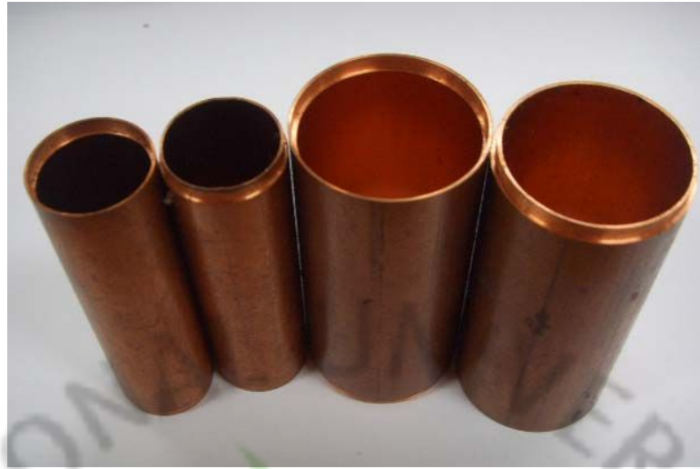
Fig. 19. The shapes of copper pipe (0.02m, 0.032m).
