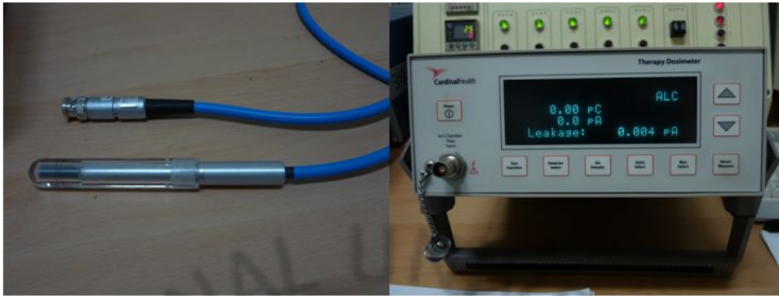
Fig. 14 Ionization chamber (PTW Freiburg) and Electrometer (Cardinal Health Co. model 35040)
