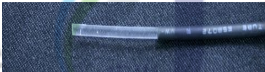
Fig. 10 Plastic optical fiber (PGR-FB3000)
