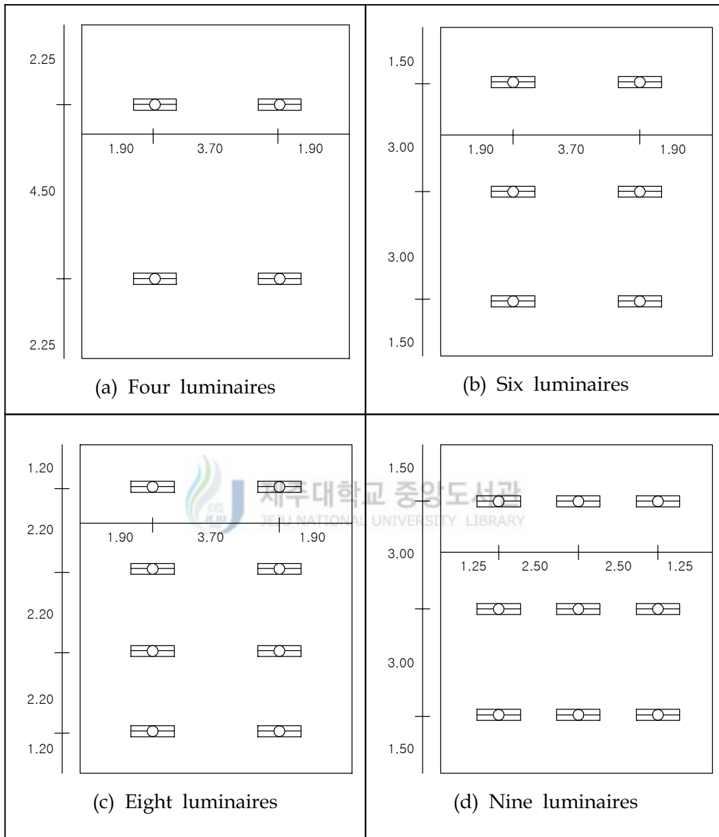
Fig. 5 Arrangement of luminaires in classroom
