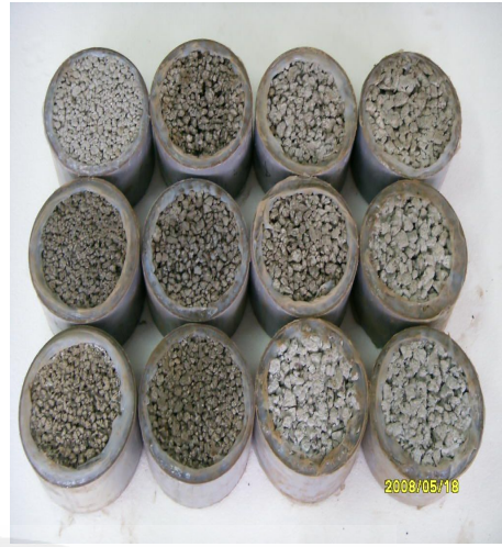
Fig. 3.12 Produced constant head permeability test apparatus Fig 3.13 The test piece of permeability test
