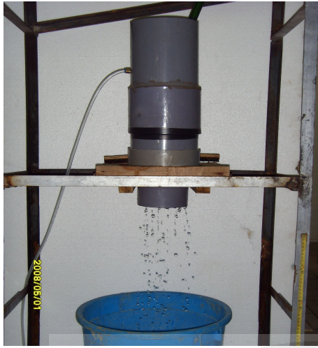
Fig. 3.12 Produced constant head permeability test apparatus Fig 3.13 The test piece of permeability test
