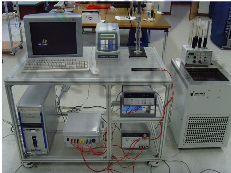
Figure. 13. The measurement experimental apparatus of thermal conductivity.
