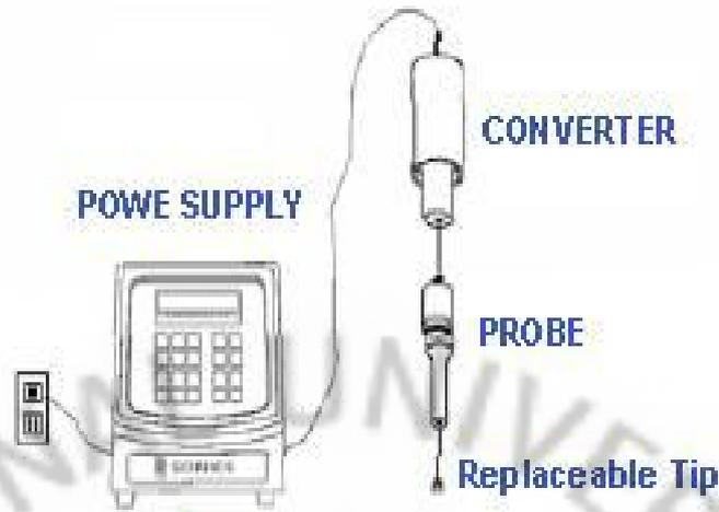
Figure. 4. Schematic diagram of the the ultrasonic dispersion(VC-505).
