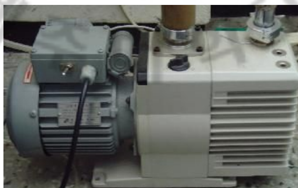
Fig. 19. Photograph of rotary pump.
