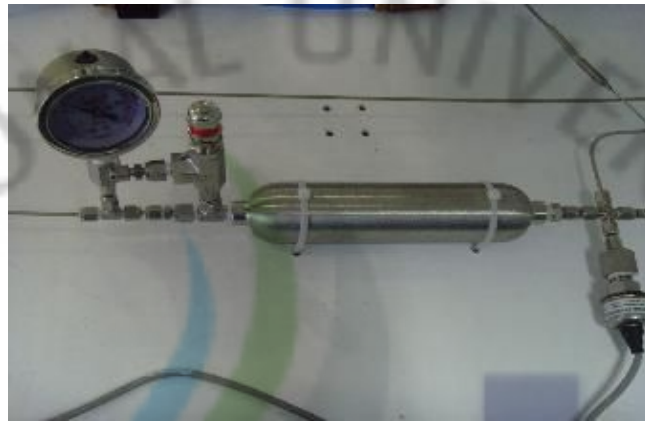
Fig. 14. Photograph of gas cylinder.
