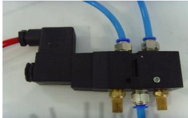
Fig. 15. Photograph of Solenoid valve.
