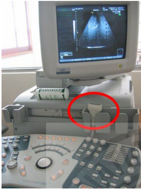
Figure 1. Ultrasonic scanner (SA-9000 PRIME, Medison, Korea) & 5-12 MHz Linear Probe used in the experiment.
