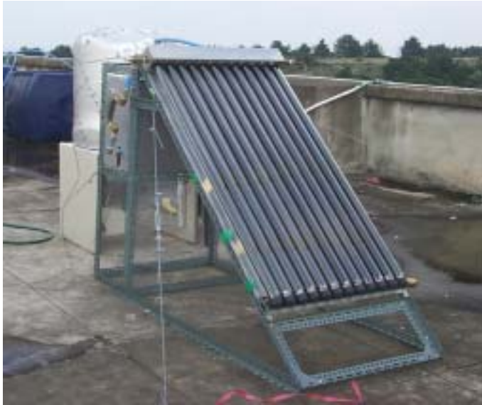
Fig. 17 Photograph of the installed all glass tube system
