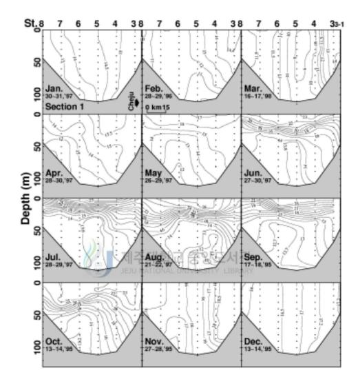
Fig. 5(A). Monthly vertical profiles of temperature between September 1995 to June 1998 in western Cheju Strait(Section1).
