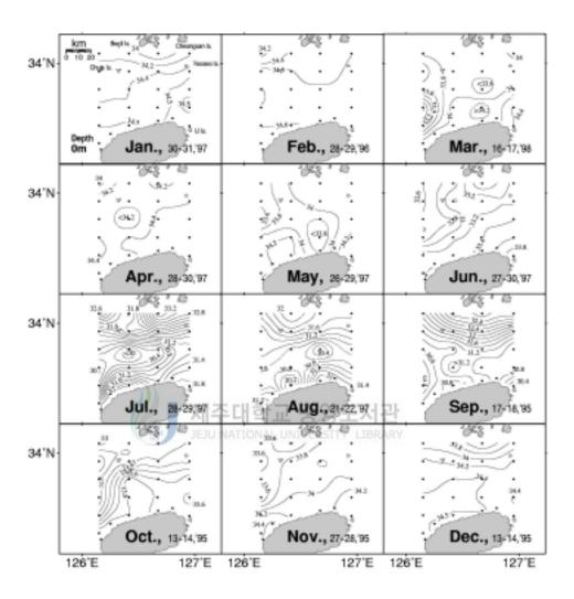
Fig. 3(B). Monthly horizontal distributions of salinity in the Cheju Strait between September 1995 to June 1998 on the depth of 0m.
