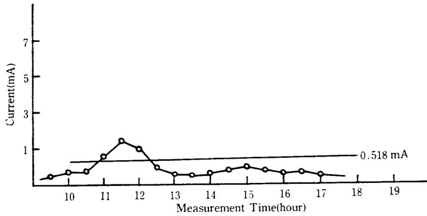
Fig. 13. A Charge Current Graph in a Rainy Day.
