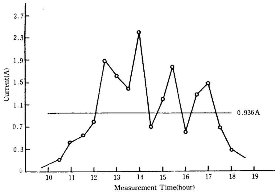
Fig. 9. A Charge Current Graph in a Fine Day.
