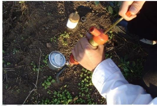
Fig. 29. Pictures of soil water sampler put into test soil and degassing the sampler to collect pore water with manual degassor.
