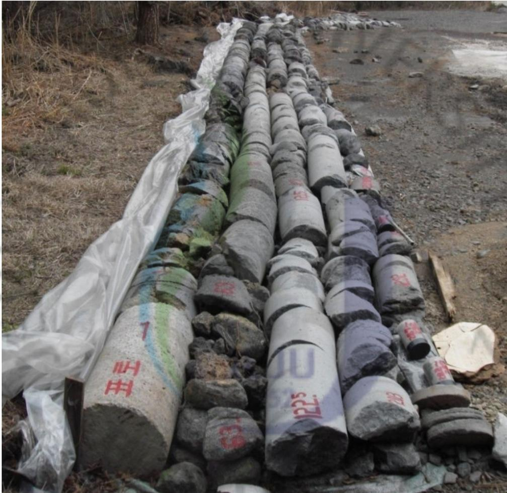
Fig. 53. Drill cores collected from the investigating bore.
