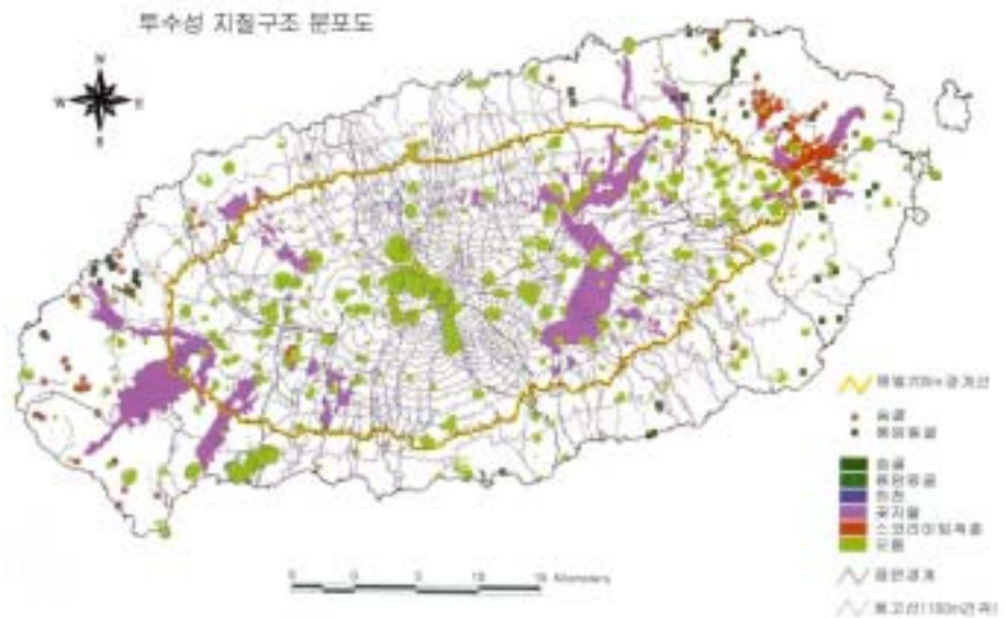
Fig. 1. Distribution map of permeable geologic structure in Jeju Island
