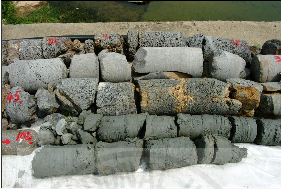
Photo 1. Drilled core showing volcanic rocks and sedimentary deposits from Kosan monitoring well.
