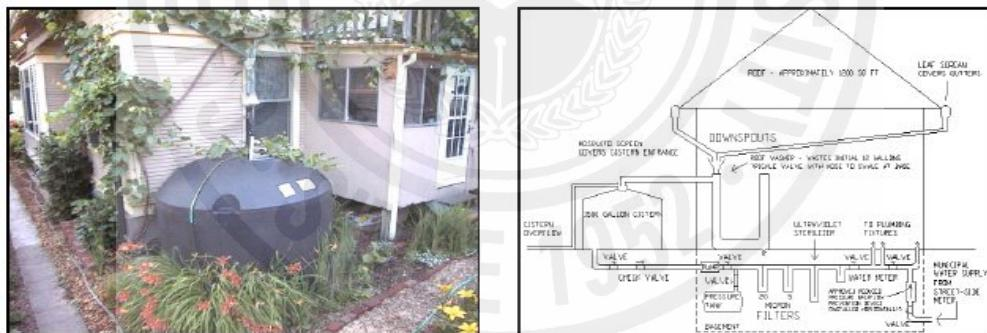
Fig. 21. Rainwater Utilization Tank and Plane Figure of Rainwater Utilization Facility in American Household
