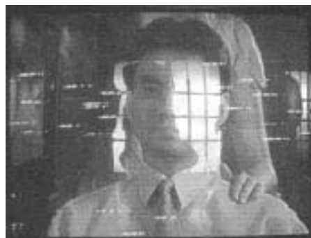
Fig. 5. Interference by the undesired signal from power line
