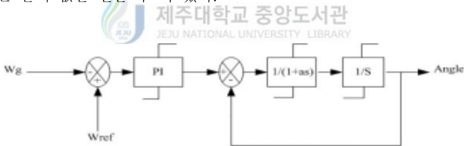
Fig. 12 Block diagram of pitch angle control
