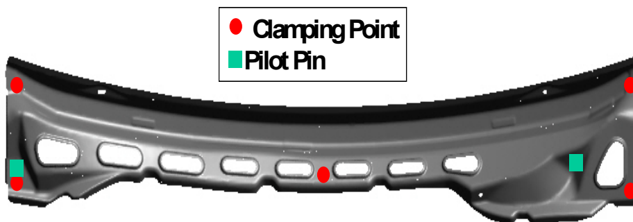
Fig. 16 Position for Pilot pin and clamping
