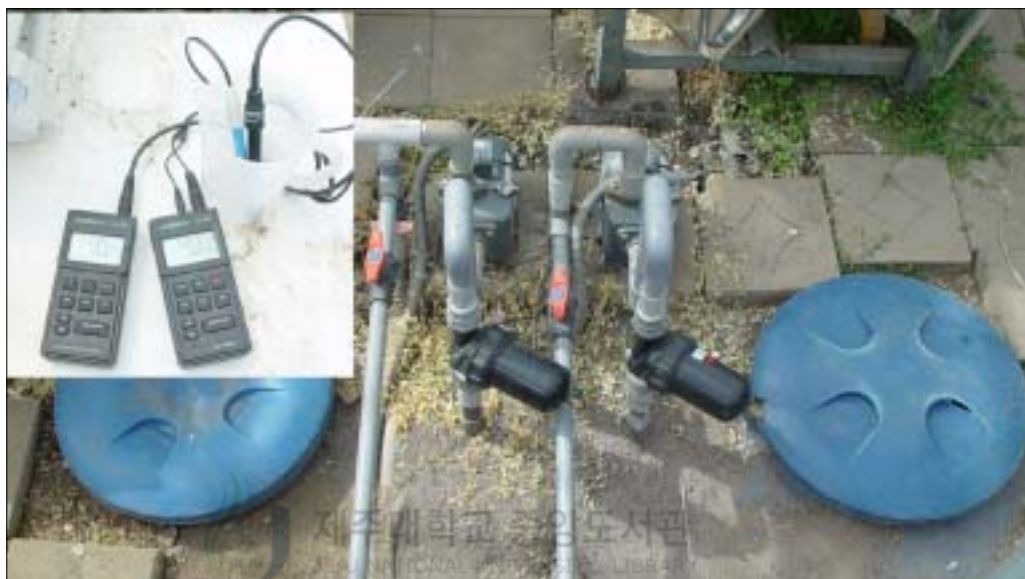
Fig. 2. Equipments for measure of pH and EC and for the supply of pump, filter and nutrient solution reservoir of aeroponic system for seed potato production used in the development of the wick hydroponic system.
