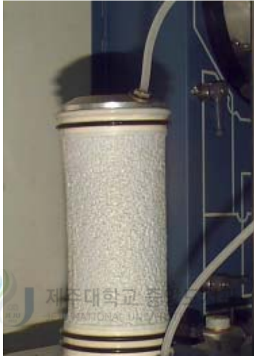
Fig 5.6 Specimen After Isotropic Test (Yellow-Brown Scoria)
