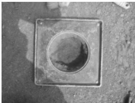
Fig 3.4 Excavation in Sand Cone Method
