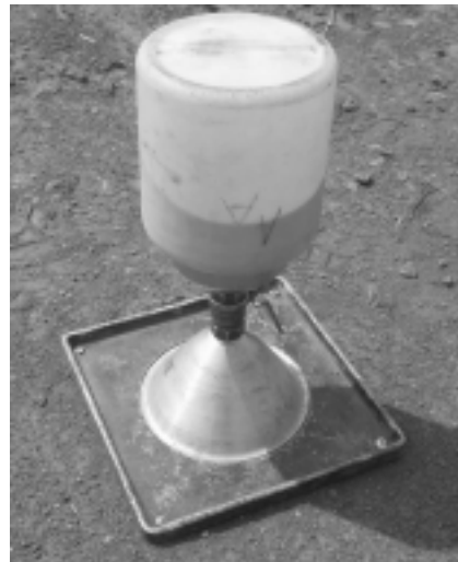
Fig 3.4 Excavation in Sand Cone Method
