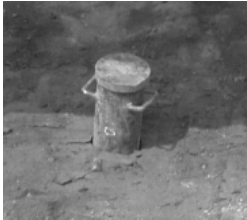
Fig 3.2 Penetration of distributed sampler
