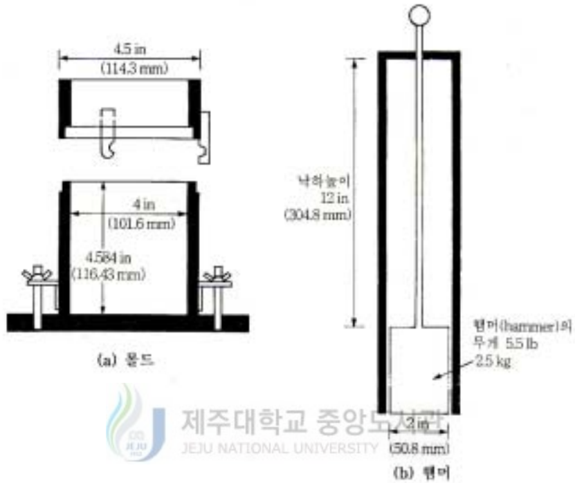
Fig. 2.13 Setup for Standard Compaction Test
