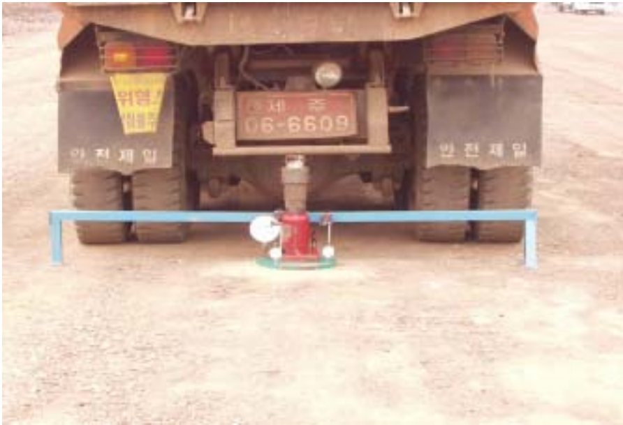
Fig. 3.2 Plate Bearing Test(Loading)
