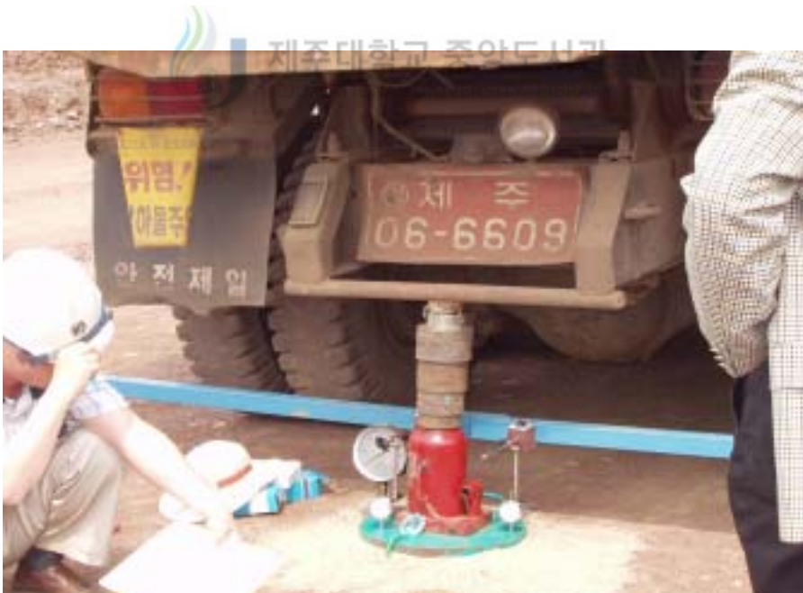
Fig. 3.3 Plate Bearing Test(Measuring Load and Settlement)
