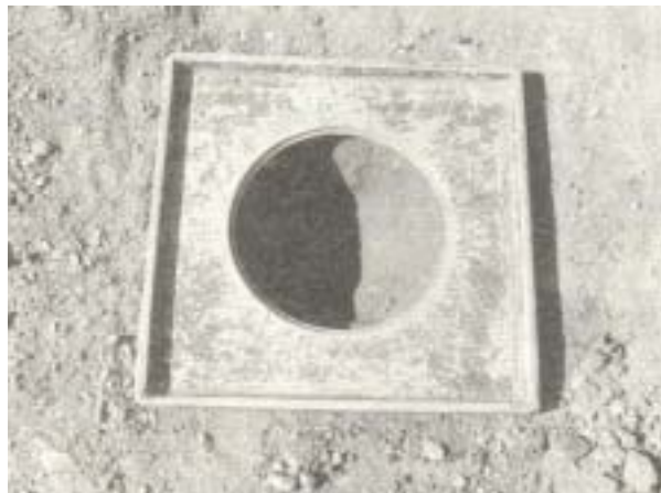
Fig. 2.28 Excavation in Sand Cone Method
