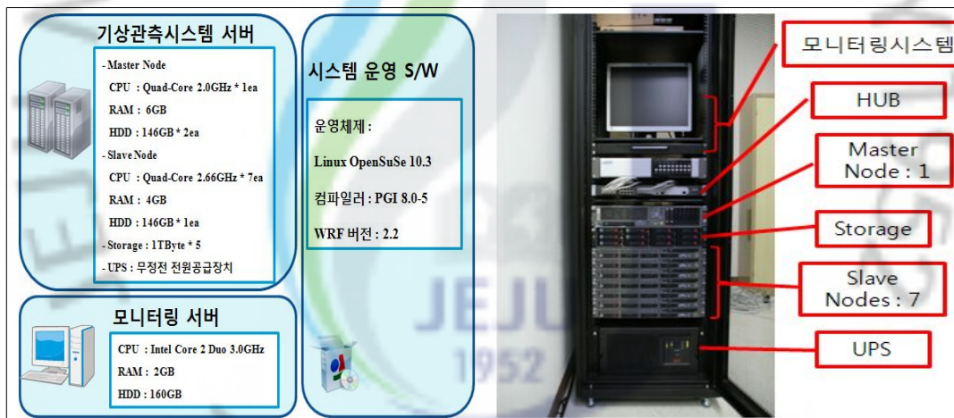
Fig. 4-1. Specification of real-time meteorological forecasting system.
