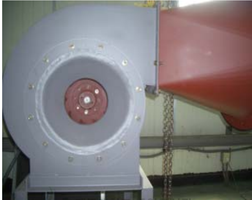
Fig. 8 View of centrifugal fan on test
