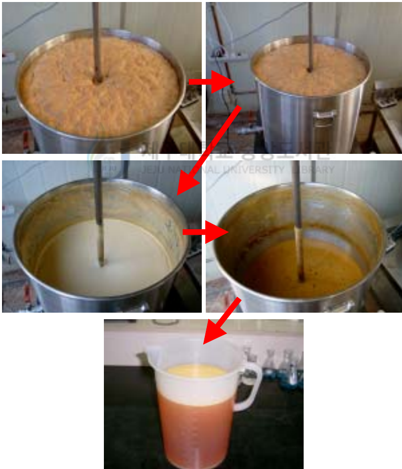
Fig. 8. The acid digestion process for liquifying bone dust.
