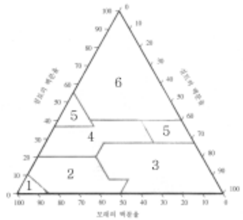
Fig 5.11 Permeability classification by soil property
