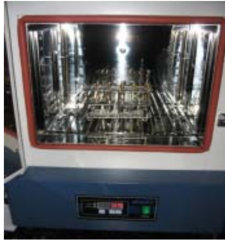
Fig. 20 The Photograph of the procedure for completing polymerization in the dry oven.
