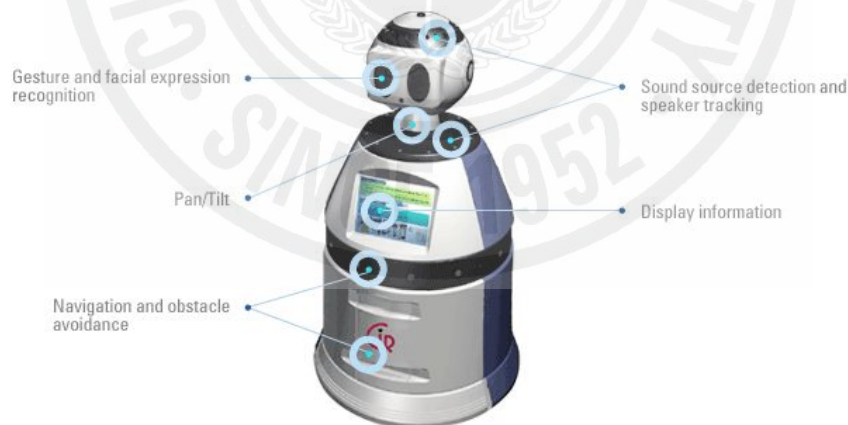
Figure 2.The Silvermate robot system and configuration
