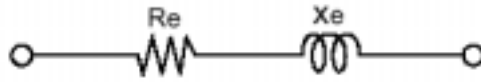
Fig. 6 Equivalent circuit of a piezoelectric ceramic resonator in the frequency band f_r \leq f \leq f_a
