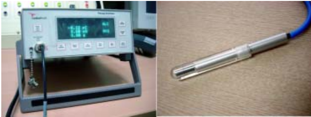
Fig 6. Electrometer and Farmer-type ionization chamber with shield cap.
