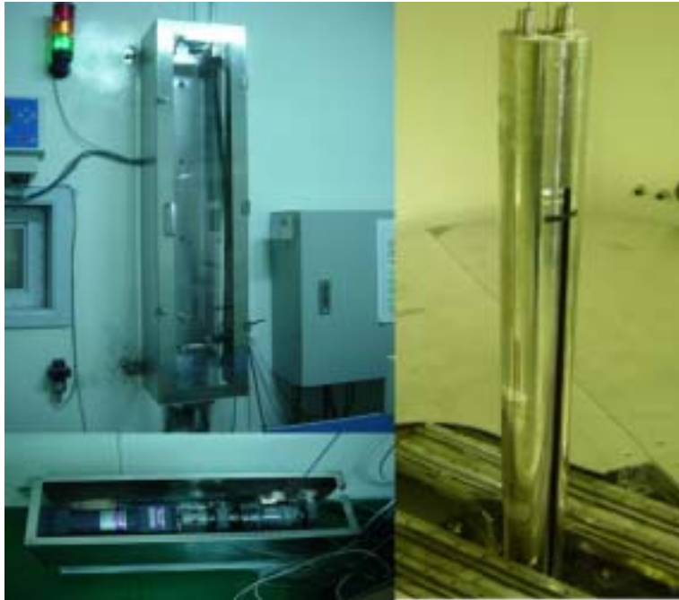
Fig 15. The running motor and control cable of the source holder
