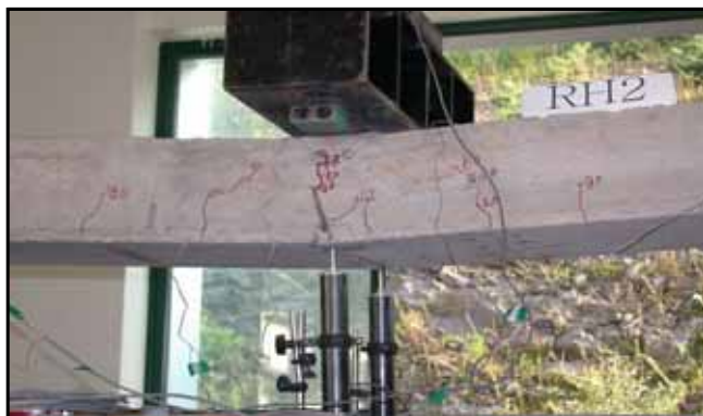
Fig. 6.10 Crack pattern of RH2 experimental specimen
