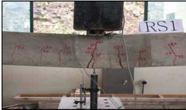
Fig. 6.8 Crack pattern of RS1 experimental specimen
