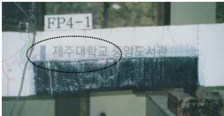
Fig. 5.16 Diagonal crack patterns of FP4-1
