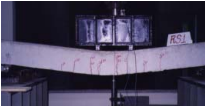
Fig. 4.7 Shear compression failure(RS1)
