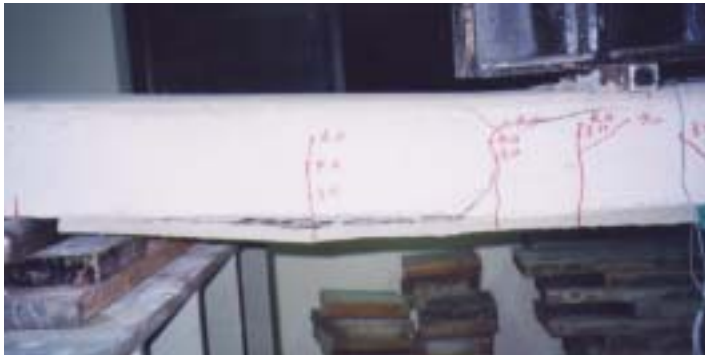
Fig. 4.10 Interfacial debonding failure(C6A-2T-2)
