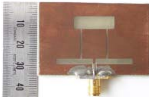
Fig. 32. Fabricated hybrid slot antenna
