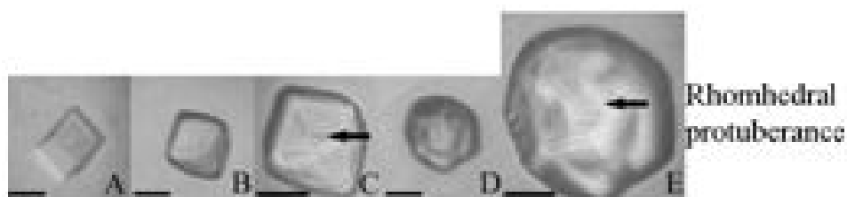
Figure 15. Light microscopic images of crystals grown in presence or absence of recombinant perlucin. (A) The control calcite crystal after incubation at 4 °C for 24 h; (B) the calcium carbonate crystal after perlucin treatment for 24 h (200 ×); (C) the calcium carbonate crystal after perlucin treatment for 24 h (400 ×); (D) the calcium carbonate crystal after perlucin treatment for 72 h (200 ×); (E) the calcium carbonate crystal after perlucin treatment for 72 h. Note the presence of recombinant perlucin rounded the edges of calcite crystals gradually and all the sharp corners disappeared after incubation for 72 h and accompanied a rhomohedral protuberance occurrence in the top of crystals, which was indicated by arrow. Scale bar: 20 μm.
