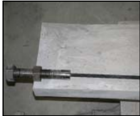
Fig 3.3(b) View of CFCC CFRP tendon and anchorage(left)
