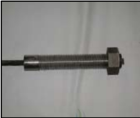
Fig 3.3(a) View of CFCC CFRP tendon and anchorage(right)
