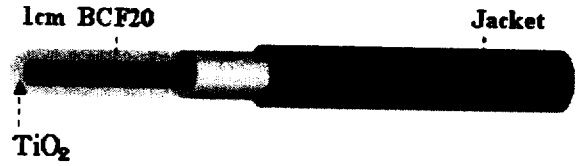
Figure 1. Fiber-optic radiation sensor tip using an organic scintillator and plastic optical fiber
